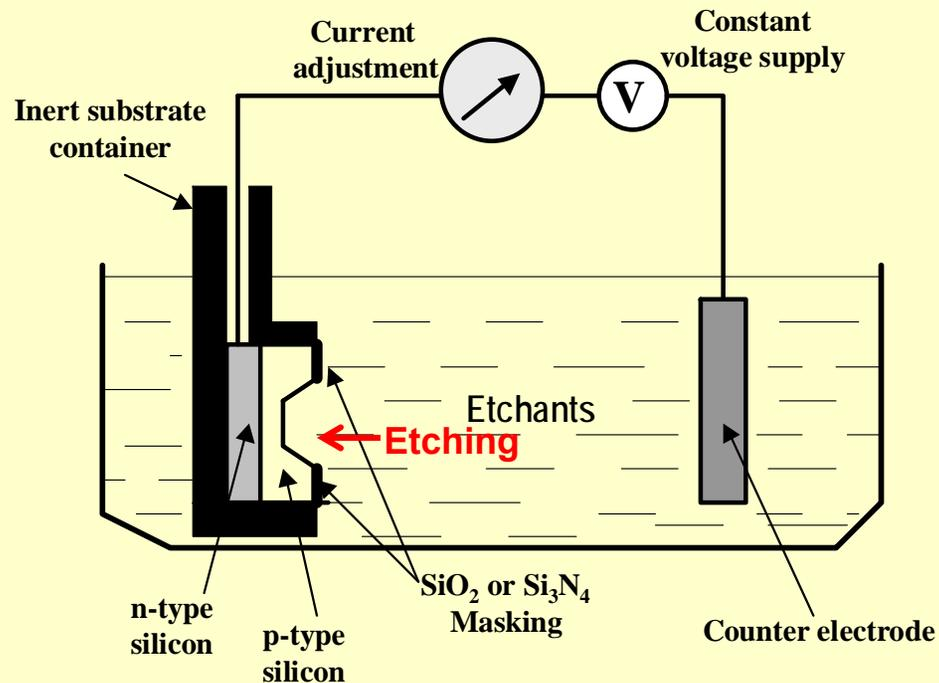
Etching stops at the interface of p- and n-type of the doped silicon.
