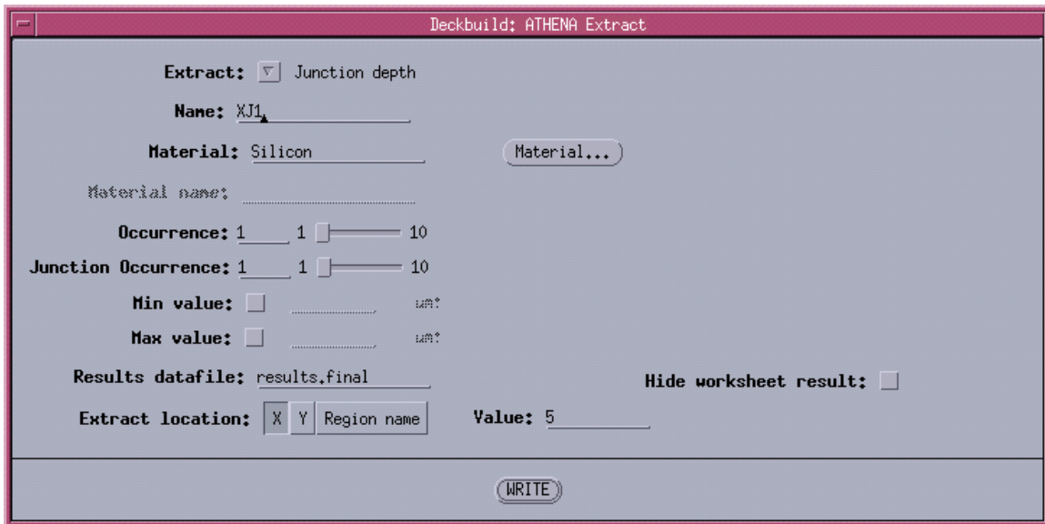
Figure 28: Extract Junction Depth.
