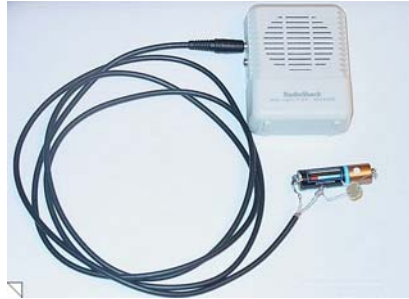
Fig. 3.1 Photoresistor receiver (powered by AA battery) and speaker/amplifier
