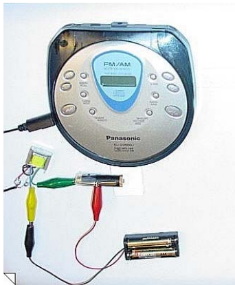
Fig. 3.3 CD player, 2-AAA batteries, battery holder, transformer, and clips
