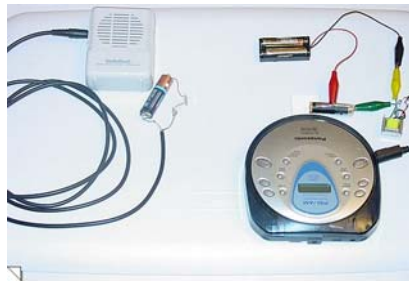
Fig. 3.2 CD player, laser transmitter, 2-AAA batteries, battery holder, transformer, clips, and receiver circuit
